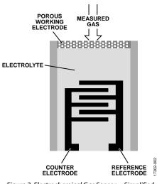
Figure 2. Electrochemical Gas Sensor—Simplified
