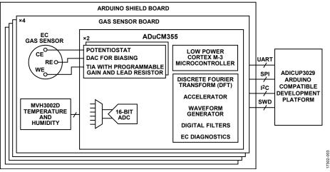
Figure 3. Simplified Circuit Block Diagram
