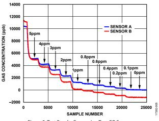
Figure 5. Test Results Comparing Two CO Sensors
