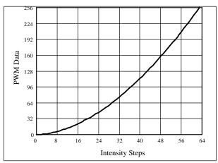
Figure 10 Gamma Correction (64 Steps)
