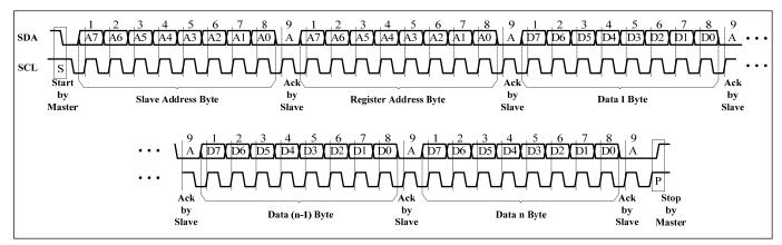
Figure 6 Writing to IS31FL3731(Automatic address increment)
