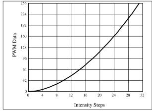
Figure 9 Gamma Correction (32 Steps)
