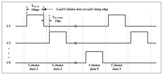
Figure 2 Scanning Timing
