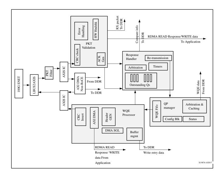
**Note:** The user logic or target IP that connects to ERNIC is referred to as application and the direction of the arrows is from master to slave.
