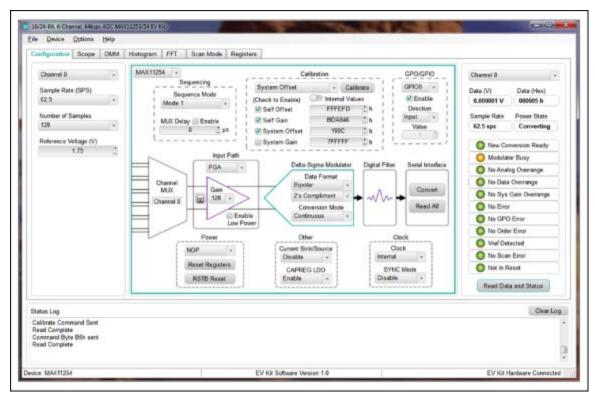
Figure 2. MAX11254 GUI setup.
