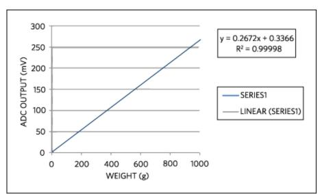
Figure 3. Transfer function of load cell.
