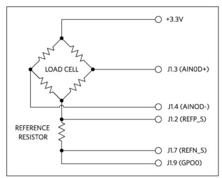
Figure 1. Weight scale Wheatstone bridge connection.
