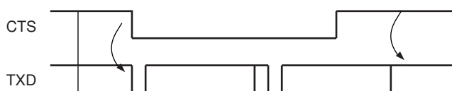
Figure 36-28. Transmitter Behavior when Operating with Hardware Handshaking
