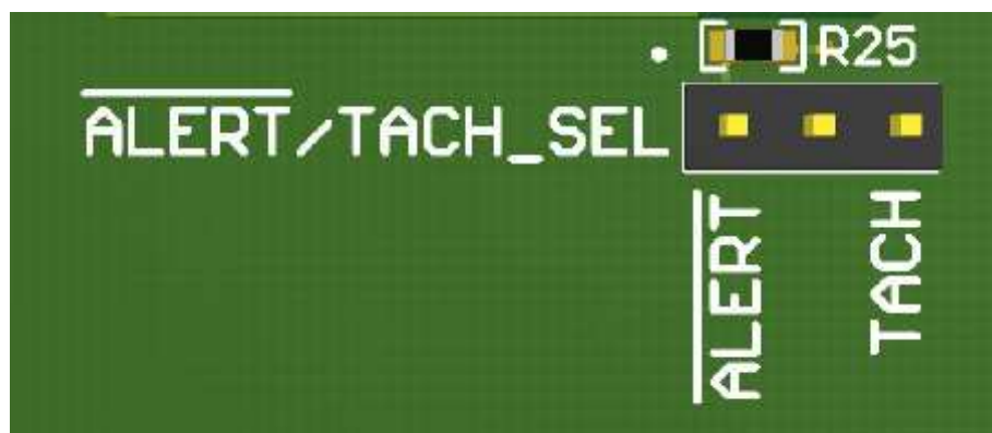
Figure 4. LM63 ALERT/TACH Select Jumper
