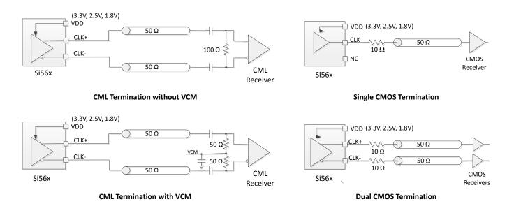
Figure 4.3. CML and CMOS Output Terminations
