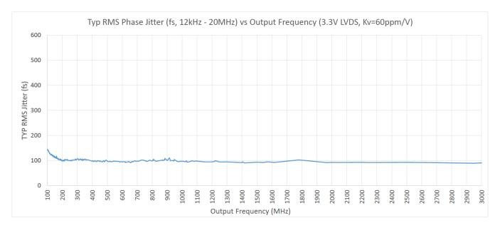
Figure 2.2. Phase Jitter vs. Output Frequency
