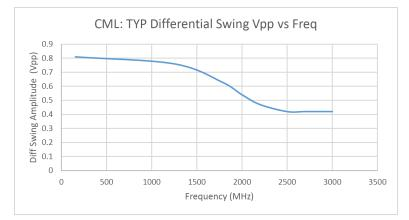
Figure 2.1. Typical Clock Output Swing Amplitudes vs. Frequency
