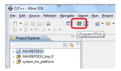
The **Program FPGA** dialog box appears. From here, an FPGA bitstream (.BIT) file is selected. Be sure to select the .BIT file by using the paths below.
