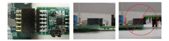
Figure 2. Pmod<sup>™</sup> Connector Alignment
