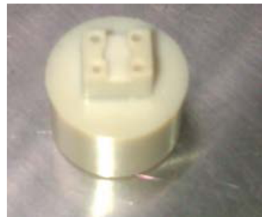
Figure 9. Recommended picker design
