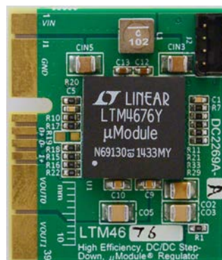
Figure 1. Dual-Output LTM4676/DC2269A-A Demo Circuit
