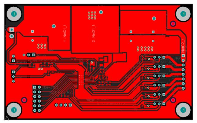
Figure 5. Top Layer Routing
