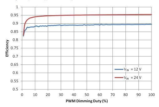
Figure 2 and Figure 3 provide typical efficiency for the TPS61196EVM-600 board.
