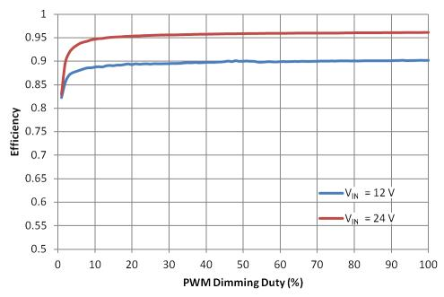
Figure 3. Efficiency Versus Dimming Cycle, 16 LEDs
