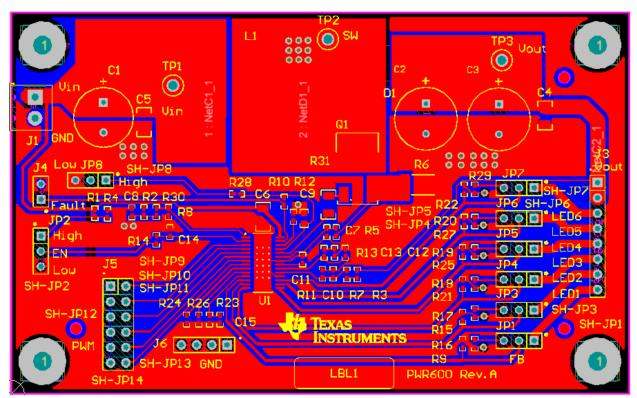
Figure 4. Top Assembly Layer
