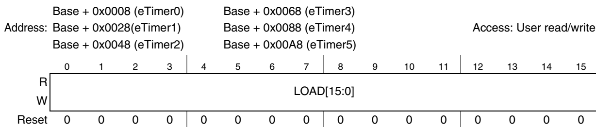
Figure 396. Load register (LOAD)
