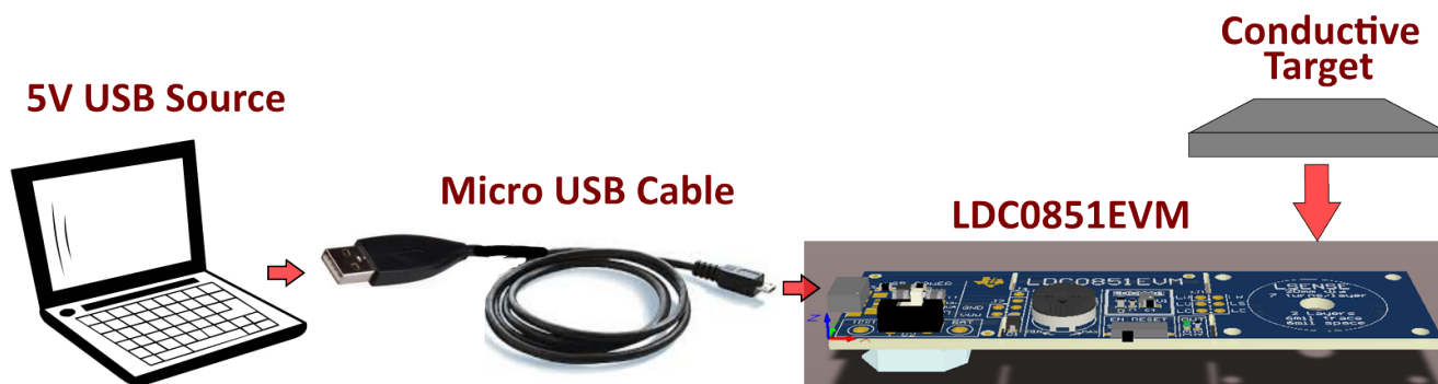
Figure 13. Insert 5-V Micro-USB
