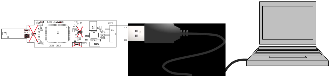
Figure 8. TMP116EVM Connection Diagram
