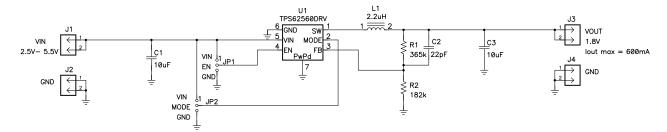
Figure 8. TPS62560EVM-330 Schematic
