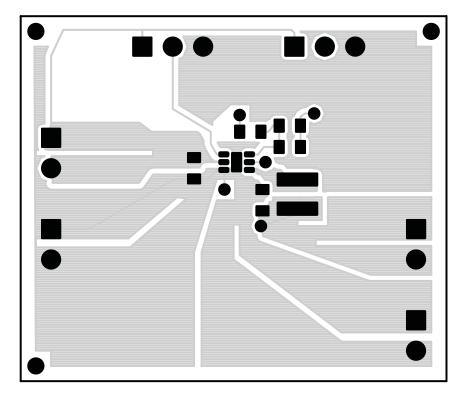
Figure 6. Top Layer Routing
