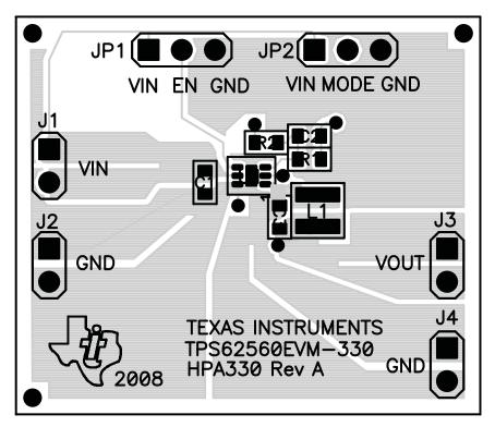
Figure 5. Assembly Layer
