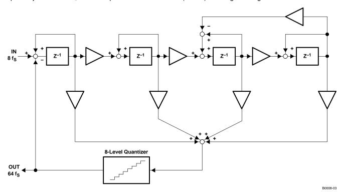
Figure 36. Eight-Level Delta-Sigma Modulator
