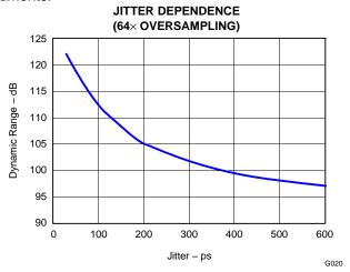
Figure 38. Jitter Sensitivity
