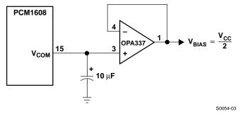
Figure 29. Biasing External Circuits Using the V<sub>COM</sub> Pin
