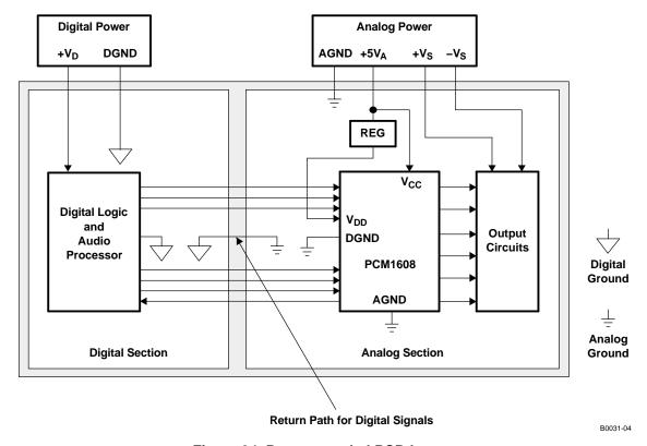
Figure 34. Recommended PCB Layout
