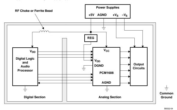
Figure 35. Single-Supply PCB Layout
