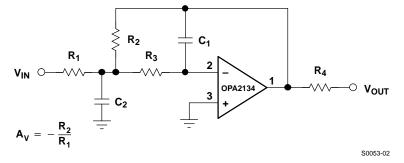
Figure 32. Dual-Supply Filter Circuit
