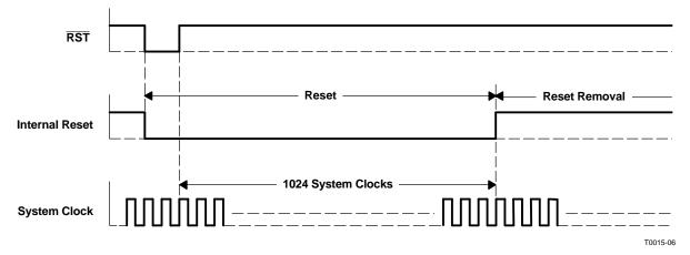
Figure 21. External Reset Timing
