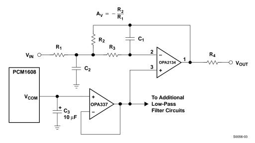
Figure 33. Single-Supply Filter Circuit
