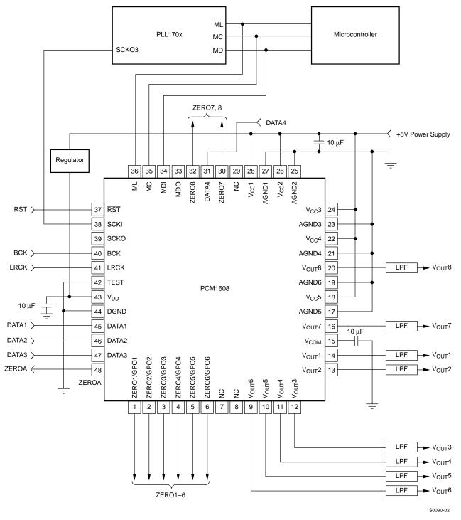
Figure 30. Basic Connection Diagram
