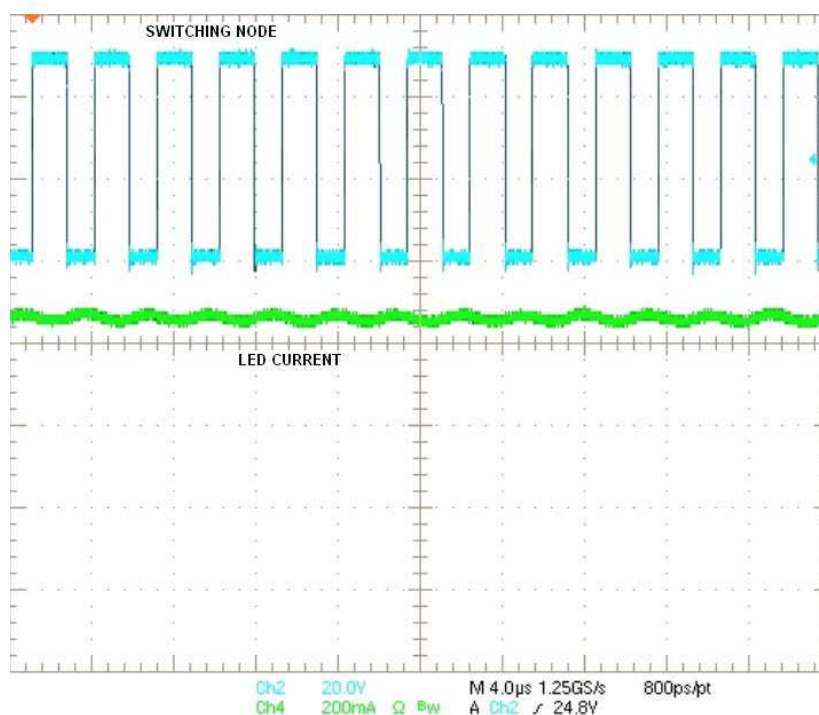
Figure 7. TPS92660EVM Buck Converter Switching Voltage and LED Current
