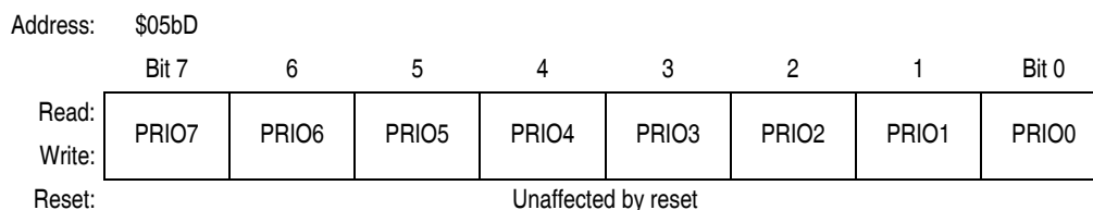
Figure 12-14. Transmit Buffer Priority Register (TBPR)
