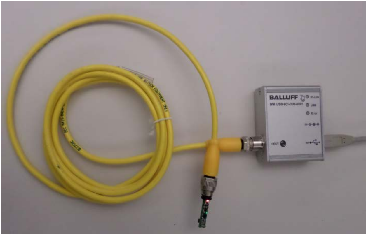
Figure 1. Santa Cruz Board Connected to a Balluff USB IO-Link Master
