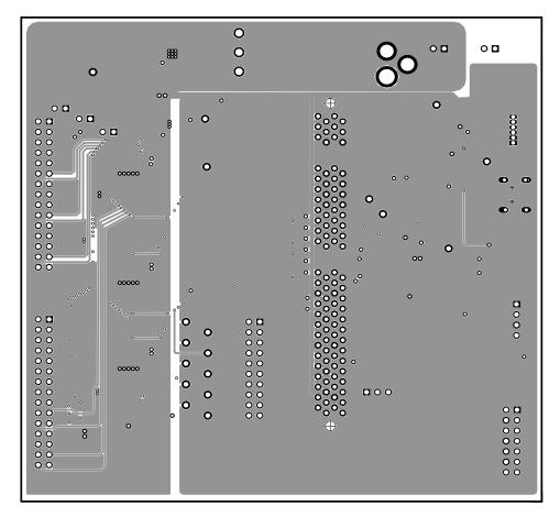
Figure 13. Bottom Layer Routing
