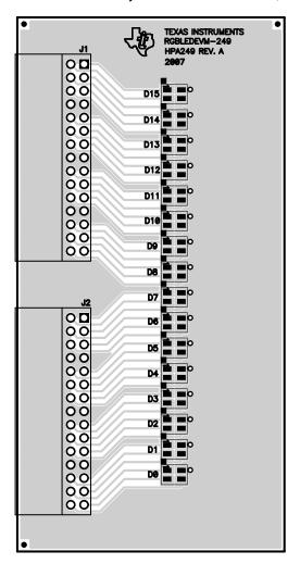
Figure 14. Assembly Layer
