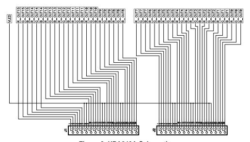
Figure 8. HPA249A Schematic
