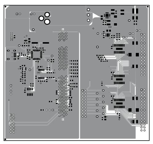
Figure 10. Top Layer Routing
