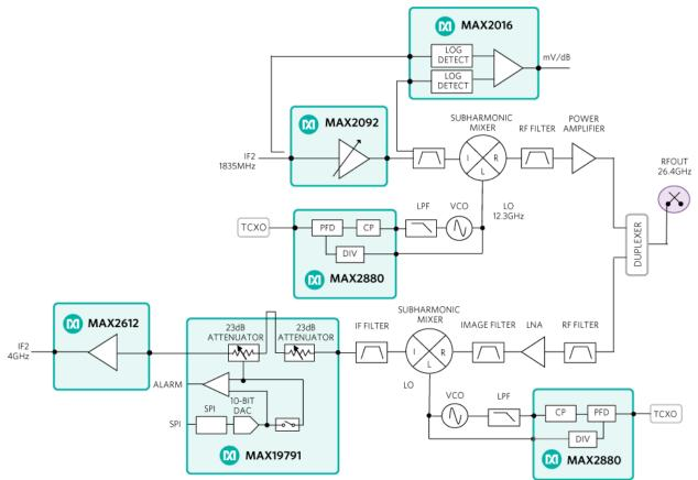
Figure 3. Schematic for the microwave up/down frequency converter section in a split mount ODU.
