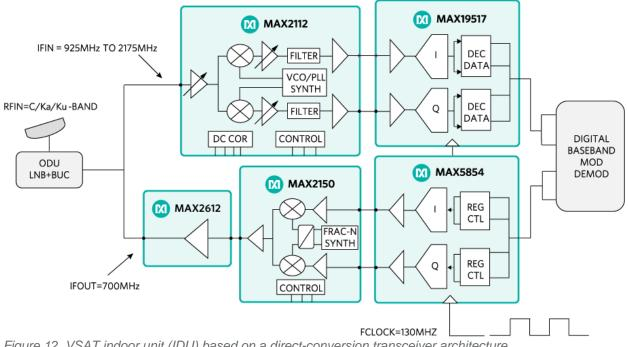
Figure 12. VSAT indoor unit (IDU) based on a direct-conversion transceiver architecture
