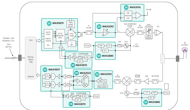
Figure 4. Schematic for a FODU RF to Bits microwave transceiver with PoE+. This radio would be encased in an environmentally hardened enclosure.
