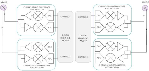
Figure 6. Spatial multiplexing with CCDP increases RF channel density.
