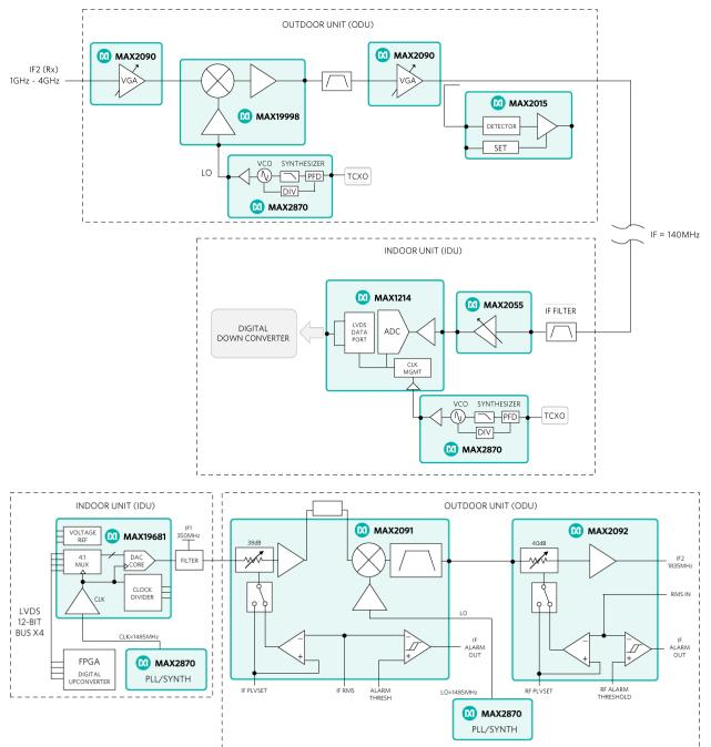
Figure 2. IF signal routing in the schematic of an SMU radio IF section. The IDU/ODU receiver (RX) is shown at the top; the IDU/ODU transmitter (TX) is at the bottom.
