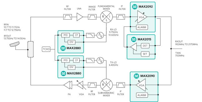
Figure 11. Analog RF building blocks play an important role in VSAT ODU microwave radios. Here the LNB and BUC rely on PLL frequency synthesizers and high-linearity VGAs for stable performance over temperature extremes.
