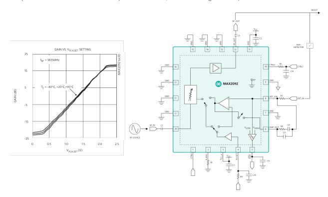
Figure 9. An important VGA feature is high linearity over a wide operating temperature range with precise linear-in-dB level control (shown in the performance curves on the left). A VGA, like the MAX2092, is a common RF building block used for ATPC applications and RX-TX signal leveling.
