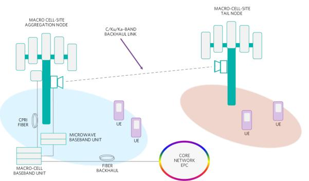
Figure 1. A PTP LOS microwave link uses a tail node and aggregation node. This approach lets remote base stations access the core network.
