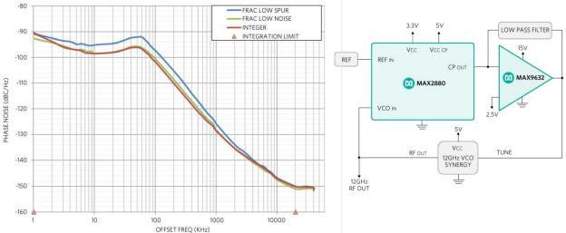
Figure 8. Phase noise is an important PLL-frequency-synthesizer performance metric in LO applications. For simplicity, passive R-C components for filtering, AC-coupling, and impedance matching are excluded at the lowpass filter for the MAX2880.
