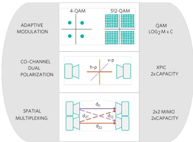
Figure 5. Three advanced digital communication techniques for increasing spectral efficiency.
