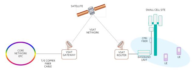
Figure 10. Satellite backhaul with a broadband VSAT system connects a remote small cell base station to the core network.
