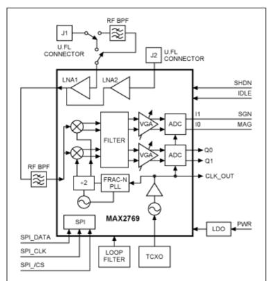
Figure 2. Block diagram for the GPS reference design.
