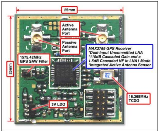
Figure 1. GPS reference design features the MAX2769.
