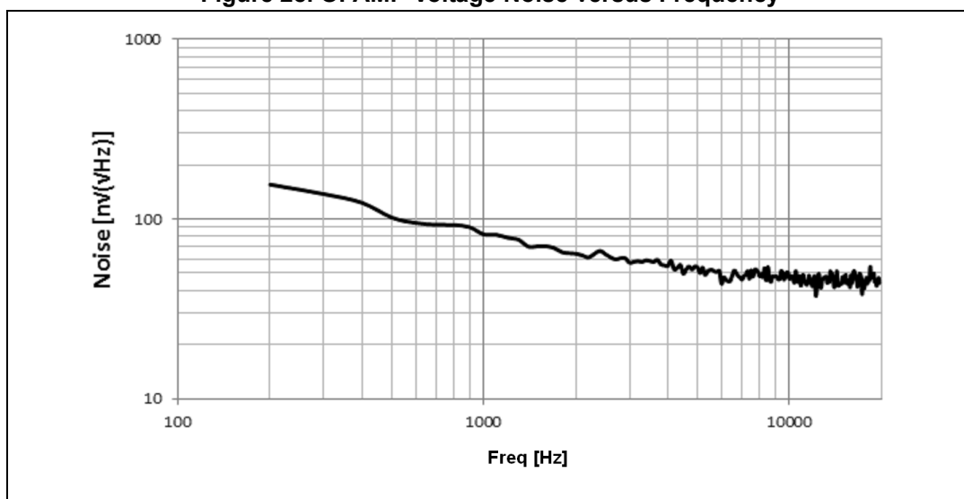
Figure 28. OPAMP Voltage Noise versus Frequency
