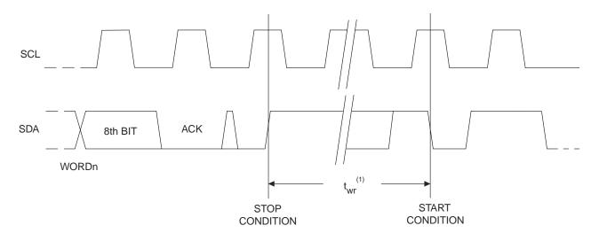
Note: The write cycle time t<sub>wr</sub> is the time from a valid stop condition of a write sequence to the end of the internal clear/write cycle
