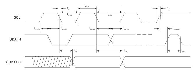
SCL: Serial Clock, SDA: Serial Data I/O
