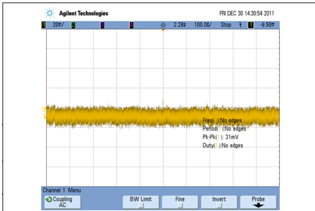
FIGURE 2-5: V_{\text{OUT}} Ripple of the Evaluation Board is less than 30 mV p-p using RC Snubber and R_{\text{BOOST}} (12V Input, 100 mA Load). Compare to Figures 2-3 and 2-4.
