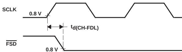
Figure 5–3. Master/Slave SCLK to \overline{FSD} Timing
