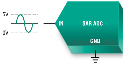
Figure 1a. Single-Ended Unipolar
