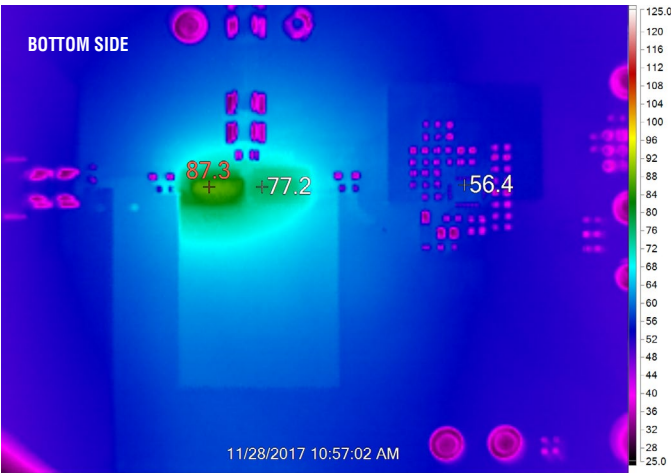
Figure 5. Thermal Performance at V_{IN} = 48V , V_{OUT} = 12V , I_{OUT} = 20A , T_A = 23^{\circ}C , in Free Air
