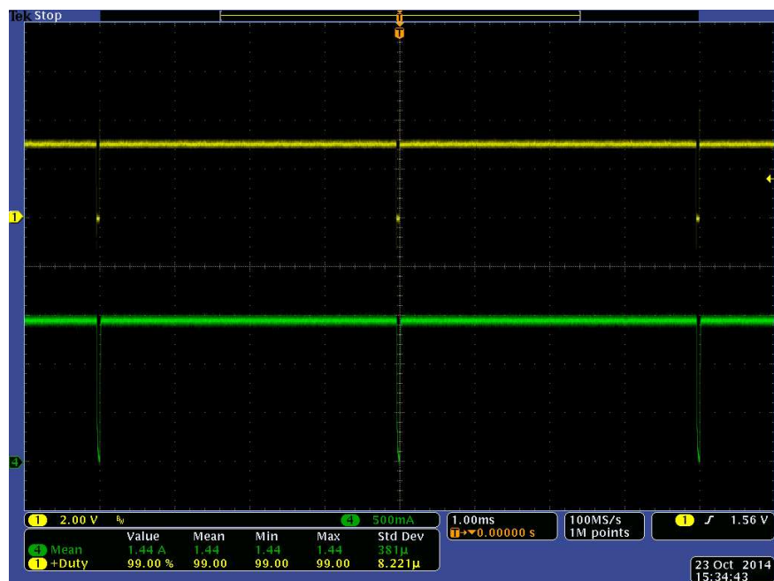
Top = PDIM Bottom = LED Current Figure 8. 99% Duty Cycle, 250-Hz PWM Dimming
