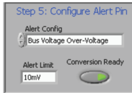
Figure 21. Configuring the Alert Pin
