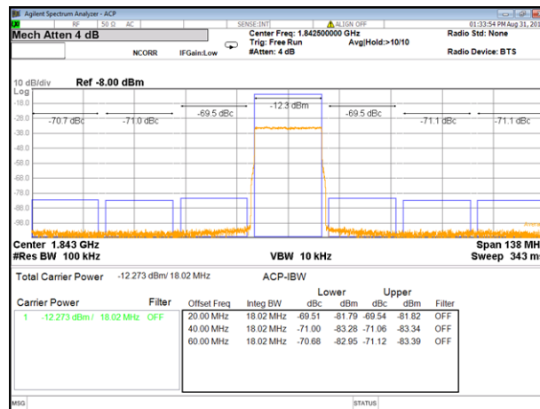
Figure 170. Dual band ACPR Performance in Downlink Band 3 with On-chip PLL
