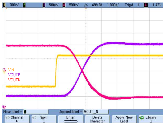
Figure 53. Step Response of the AMC1300
