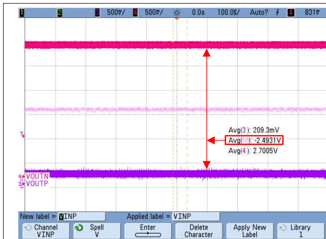
Figure 49. Typical Negative Clipping Output of the AMC1300
