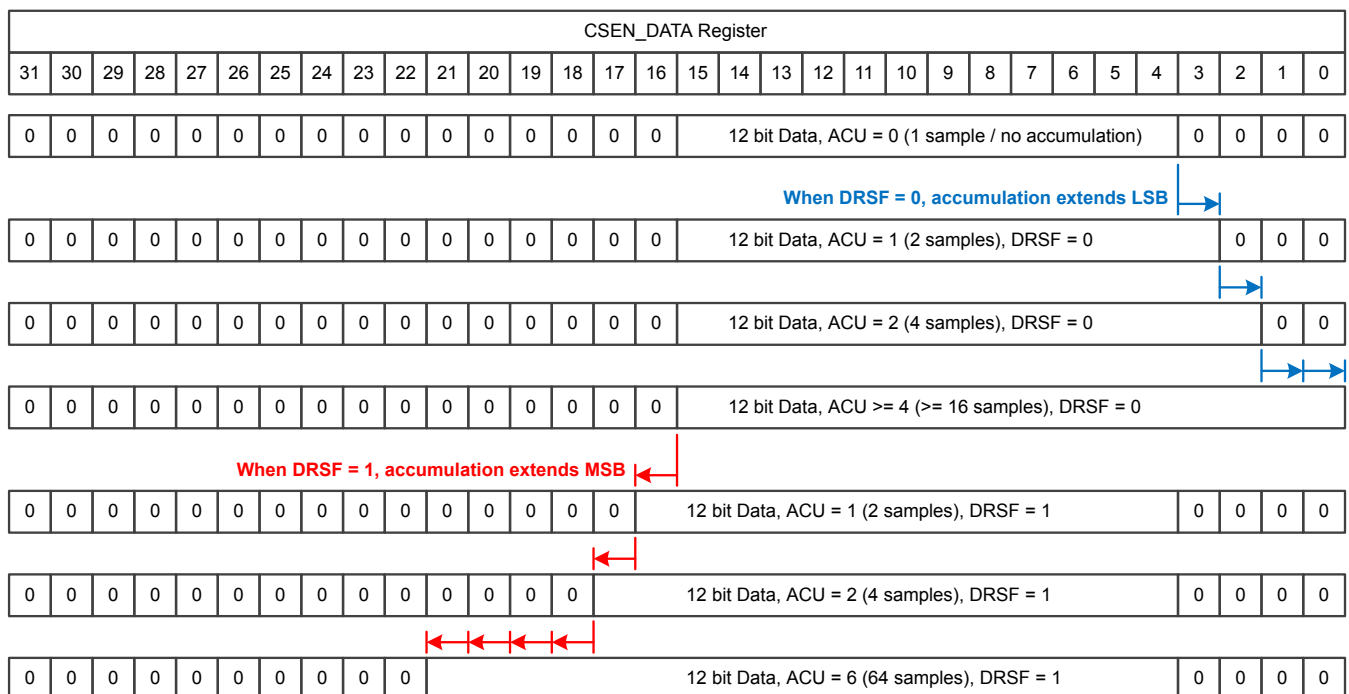
Figure 41.7. Data Encoding for Different Accumulator Settings
