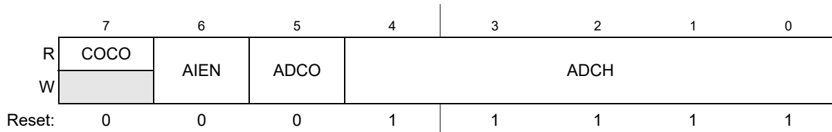
Figure 10-2. Status and Control Register (ADCSC1)
