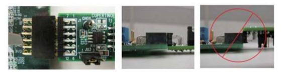
Figure 2. Pmod<sup>™</sup> Connector Alignment
