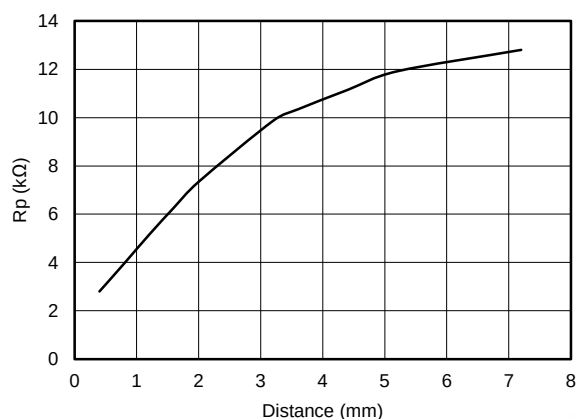
Figure 9. Typical R_p vs Distance With 14mm PCB Coil
