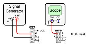
Figure 4. Example for Stimulus and Probe Points with JMP4 and JMP14
