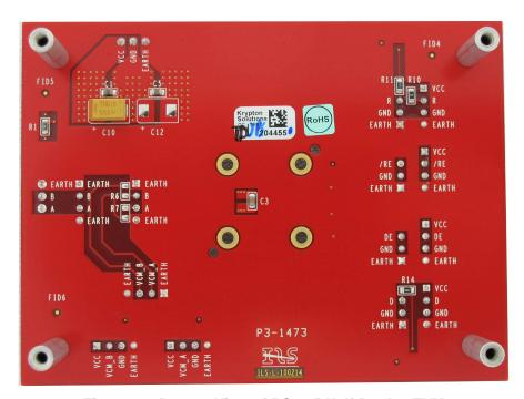
Figure 11. Bottom View of RS-485 Half-Duplex EVM
