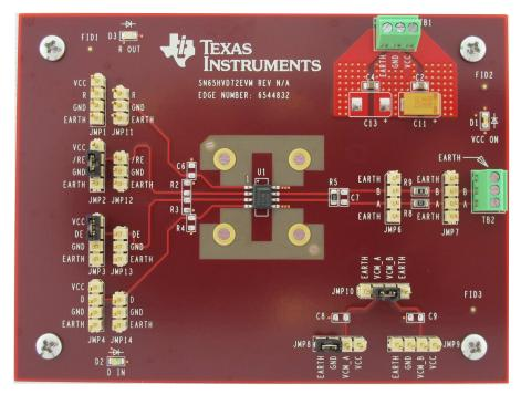
Figure 10. Top View of RS-485 Half-Duplex EVM
