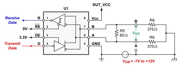
Figure 7. Configuration for Maximum Loading
