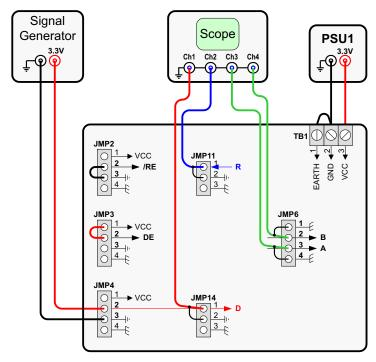
Figure 6. RS-485 Half-Duplex EVM Setup for Normal Transceiver Operation
