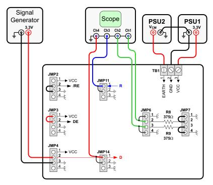
Figure 8. RS-485 Half-Duplex EVM Setup for Maximum Loading
