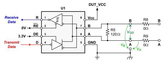
Figure 5. Transceiver Configuration for Normal Operation
