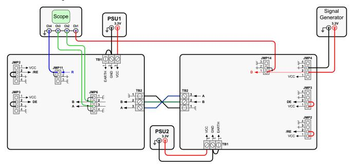
Figure 9. RS-485 Half-Duplex EVM Configurations: Left as Receiver EVM, Right as Transmitter EVM
