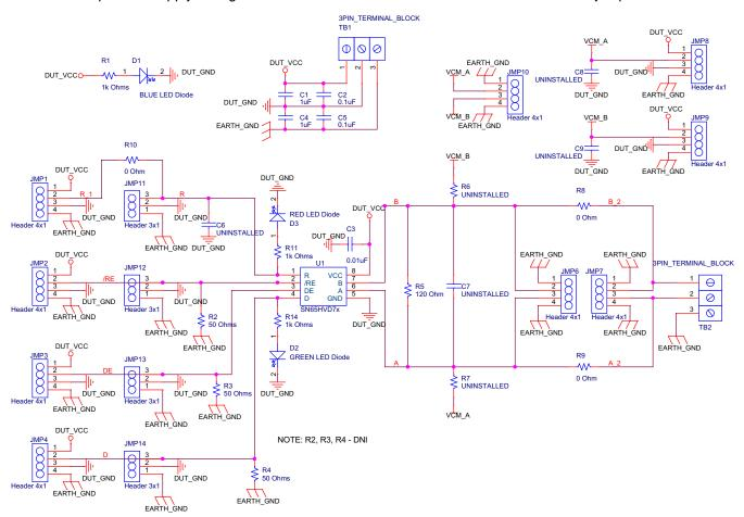
Figure 2. RS-485 Half-Duplex EVM Schematic
