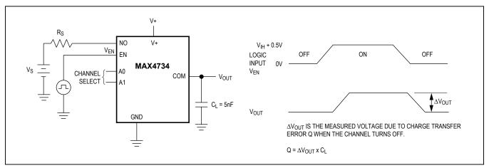
Figure 3. Charge Injection
