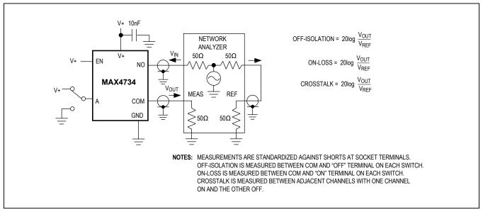
Figure 5. Off-Isolation/On-Channel/Crosstalk Bandwidth
