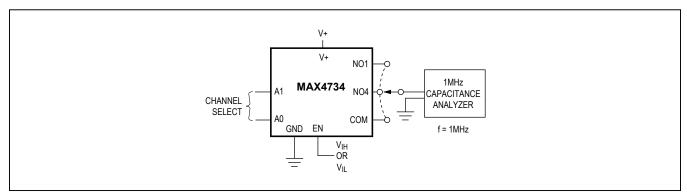
Figure 4. Channel Off/On-Capacitance
