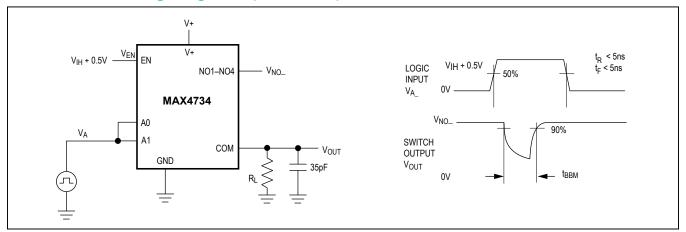
Figure 2. Break-Before-Make Interval
