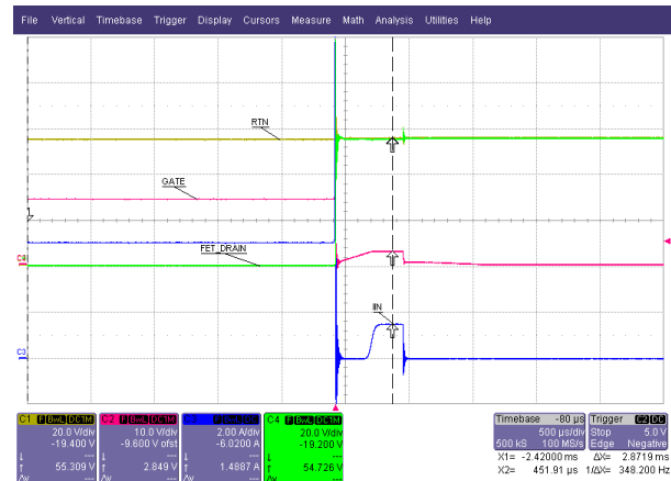
Scope GND = -48V_B, 5-A Load, After Inductor
