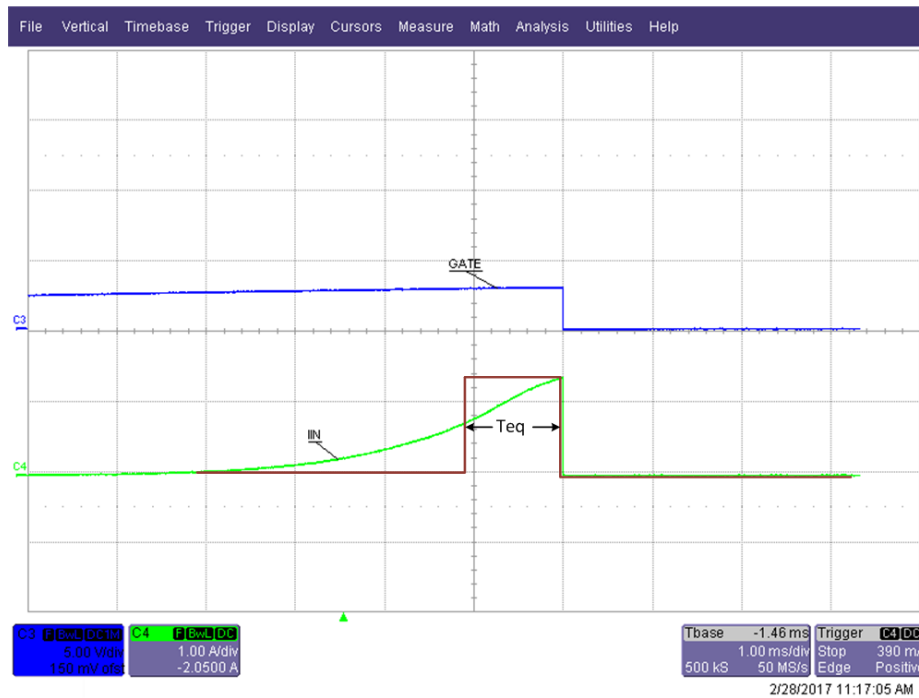
Figure 13. Teq During a Start Into a Short
