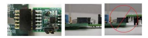
Figure 2. Pmod™ Connector Alignment
