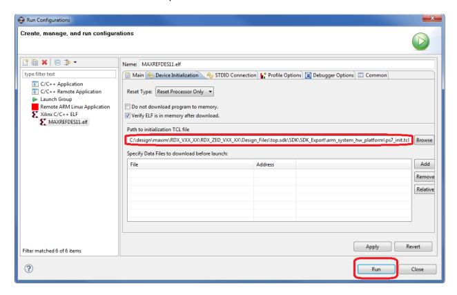
Once the Debug/MAXREFDES6 configuration is set up once, you just need to press the **Run** button if you ever want to run the program again.
