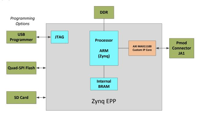
Figure 3. Block Diagram of FPGA Hardware Design
