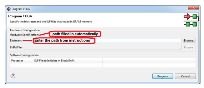
It takes approximately 10 seconds to download the FPGA, then a message box indicating **FPGA configuration complete** appears.
