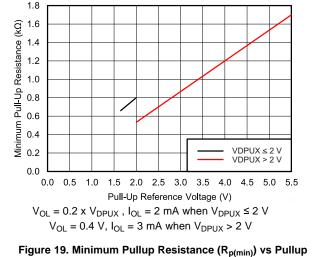
Figure 19. Minimum Pullup Resistance (R<sub>p(min)</sub>) vs Pullu<sub>l</sub> Reference Voltage (V<sub>DPUX</sub>)
