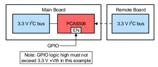
Figure 9. An example of connecting a remote board to a main board (backplane)
