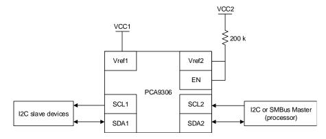
Figure 12. Master on side 2 of PCA9306
