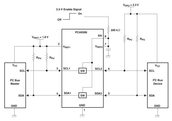
Figure 17. Typical Application Circuit (Switch Enable Control)
