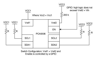
Figure 10. Switch Configuration
