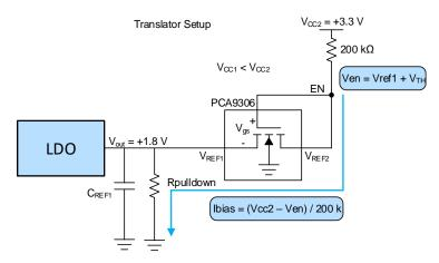
Figure 14. Example with Leakage current path when using an LDO
