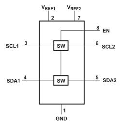
Figure 15. Block Diagram of PCA9306
