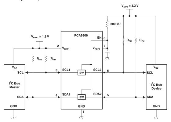
Figure 16. Typical Application Circuit (Switch Always Enabled)
