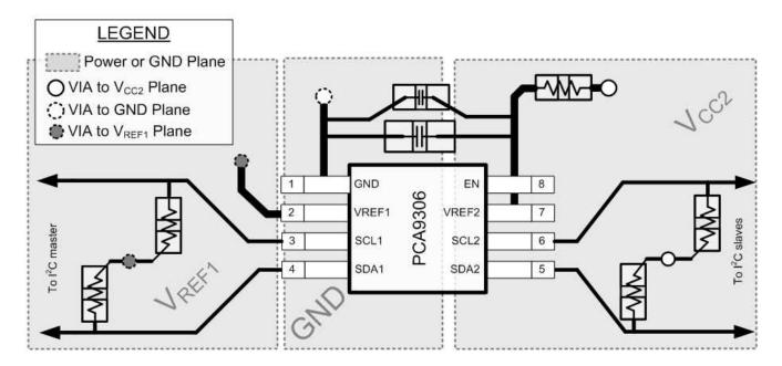
Figure 20. PCA9306 Layout Example
