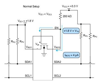
Figure 6. Normal Setup
