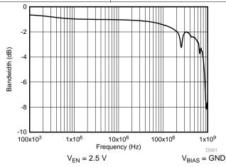
Figure 3. Typical Bandwidth of PCA9306
