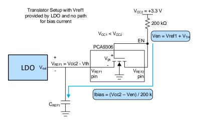
Figure 13. Example of no leakage current path when using LDO
