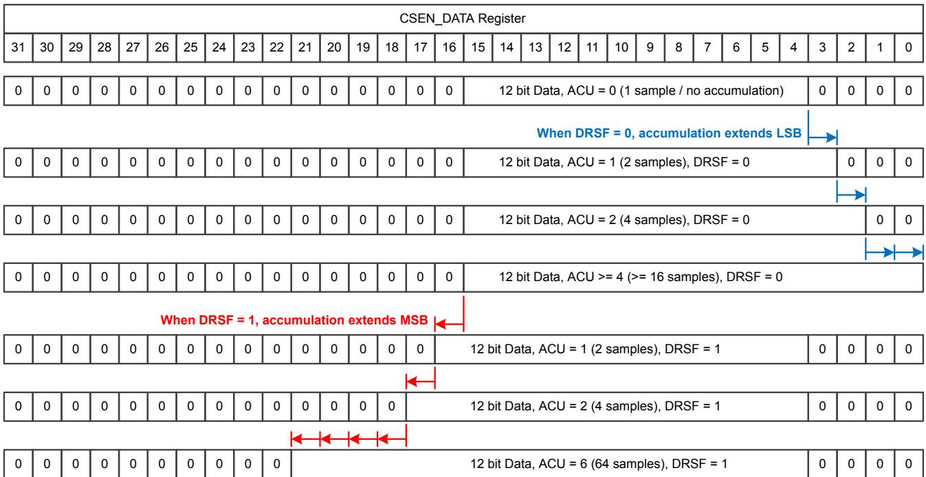
Figure 34.7. Data Encoding for Different Accumulator Settings
