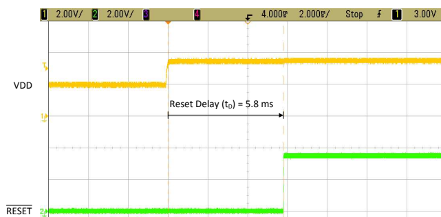
Figure 16. TPS3840EVM RESET Delay Time ( t_D ) with C_T Tied to GND Through 0.01- \mu F Capacitor
