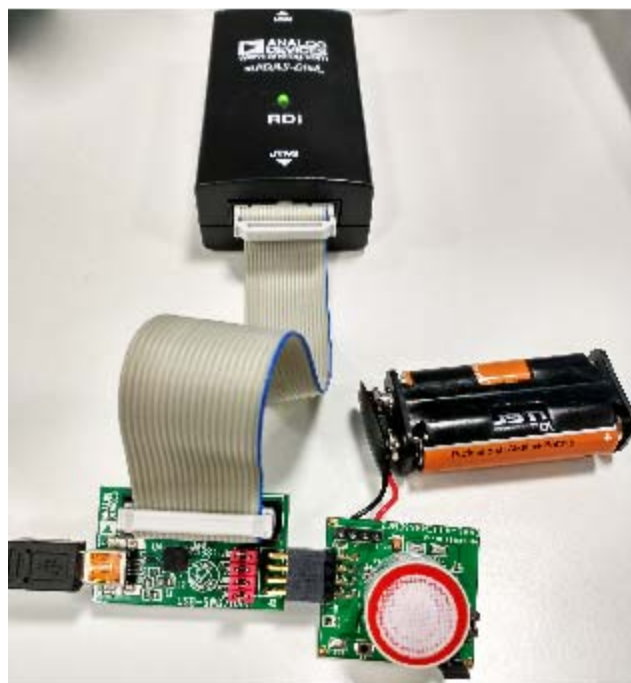
Figure 9. Connecting Programming/Debugging POD to the EVAL-ADuCM355EMCZ
