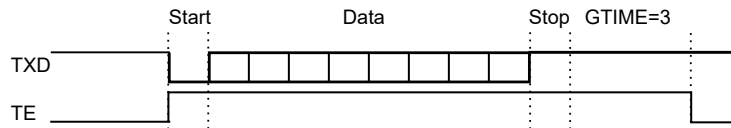
Figure 31-15. Example of TE Drive with Guard Time
