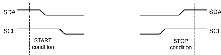
Figure 14-3. START and STOP Conditions
