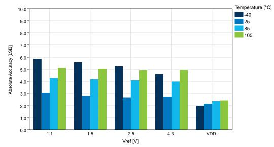
Figure 35-43. Absolute Accuracy vs. V<sub>ref</sub> (V<sub>DD</sub>=5.0V, 115ksps)
