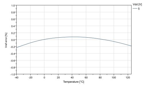
Figure 35-35. Internal 4.3V Reference vs. Temperature
