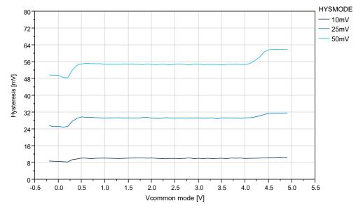
Figure 35-53. Hysteresis vs.  $V_{CM}$  - 10mV to 50mV ( $V_{DD}$ =5V, T=25°C)
