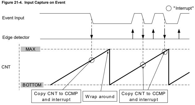
It is recommended to write zero to the TCB.CNT register when entering this mode from any other mode.
