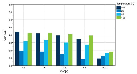
Figure 35-47. Gain Error vs. V<sub>ref</sub> (V<sub>DD</sub>=5.0V, 115ksps)
