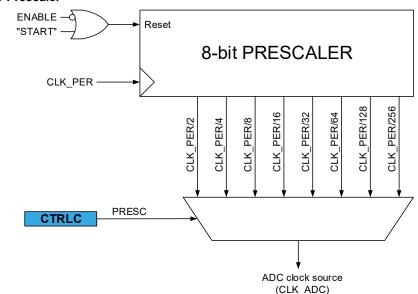
The ADC requires an input clock frequency between 50kHz and 1.5MHz for maximum resolution. If a lower resolution than 10 bits is selected, the input clock frequency to the ADC can be higher than 1.5MHz to get a higher sample rate.
