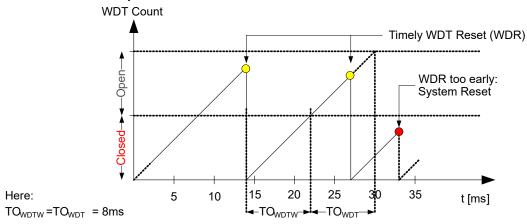
The window mode is enabled by writing a non-zero value to the WINDOW bit field in the Control A register (WDT.CTRLA), and disabled by writing WINDOW=0x0.
