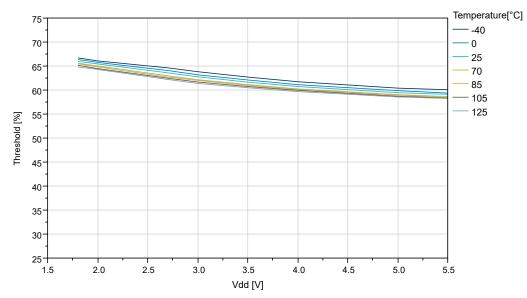
Figure 35-19. IO Pin Input Threshold Voltage vs. V<sub>DD</sub> (V<sub>IH</sub>)
