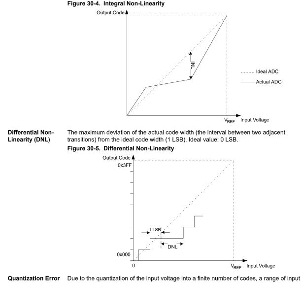
**Quantization Error** Due to the quantization of the input voltage into a finite number of codes, a range of input voltages (1 LSB wide) will code to the same value. Always ±0.5 LSB.
