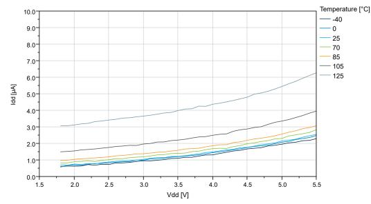
Figure 35-13. Standby Mode Supply Current vs. V<sub>DD</sub> (RTC running with internal OSCULP32K)
