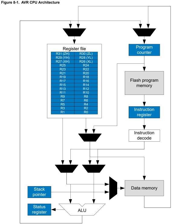
The Arithmetic Logic Unit (ALU) supports arithmetic and logic operations between registers or between a constant and a register. Single-register operations can also be executed in the ALU. After an arithmetic operation, the status register is updated to reflect information about the result of the operation.
