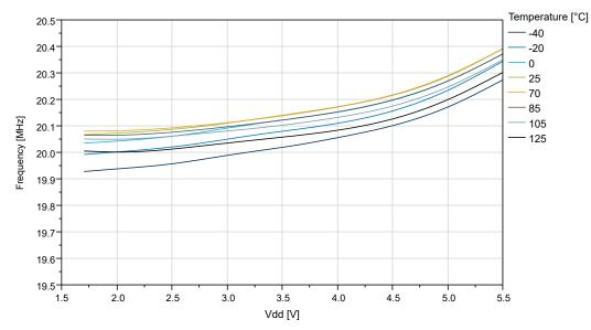
Figure 35-59. OSC20M Internal Oscillator: Frequency vs. V<sub>DD</sub>
