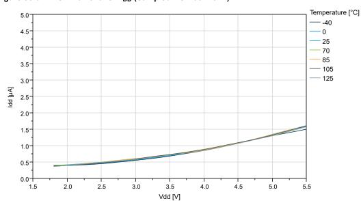
Figure 35-37. BOD Current vs. V<sub>DD</sub> (Sampled BOD at 125Hz)
