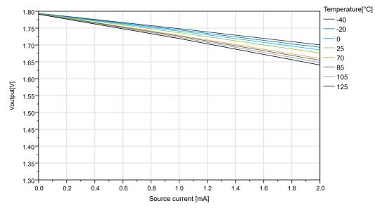
Figure 35-25. IO Pin Output Voltage vs. Source Current (V<sub>DD</sub>=1.8V)
