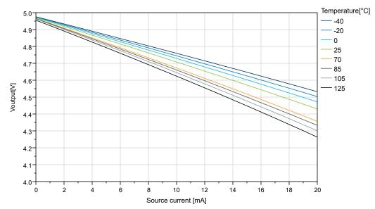
Figure 35-27. IO Pin Output Voltage vs. Source Current (V<sub>DD</sub>=5.0V)
