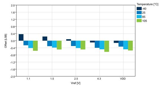
Figure 35-51. Offset Error vs. V<sub>ref</sub> (V<sub>DD</sub>=5.0V, 115ksps)
