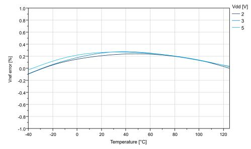
Figure 35-33. Internal 1.1V Reference vs. Temperature
