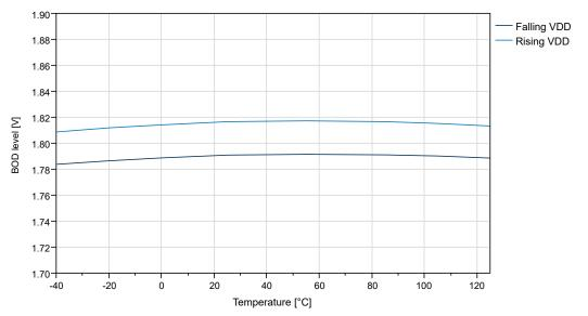
Figure 35-40. BOD Threshold vs. Temperature (Level 2.6V)
