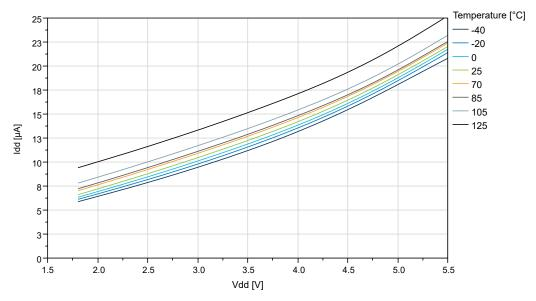
Figure 35-5. : Active Supply Current vs. V<sub>DD</sub> (f=32KHz OSCULP32K)
