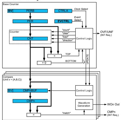
Figure 20-2. Timer/Counter Block Diagram
