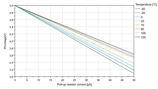
Figure 35-31. IO Pin Pull-Up Resistor Current vs. Input Voltage (V<sub>DD</sub>=5.0V)
