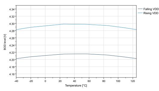
Figure 35-41. BOD Threshold vs. Temperature (Level 4.3V)
