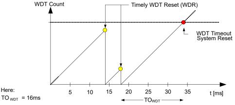
Normal mode is enabled as long as the WINDOW bit field in the Control A register (WDT.CTRLA) is 0x0.
