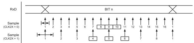
Figure 24-8. Sampling of Data and Parity Bits
