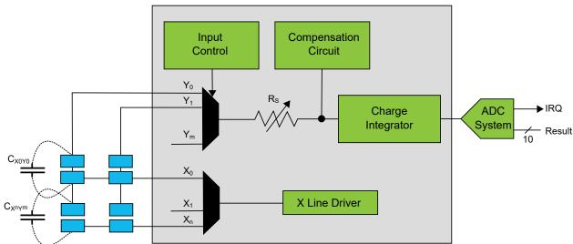
Figure 32-2. PTC Block Diagram Self-Capacitance
