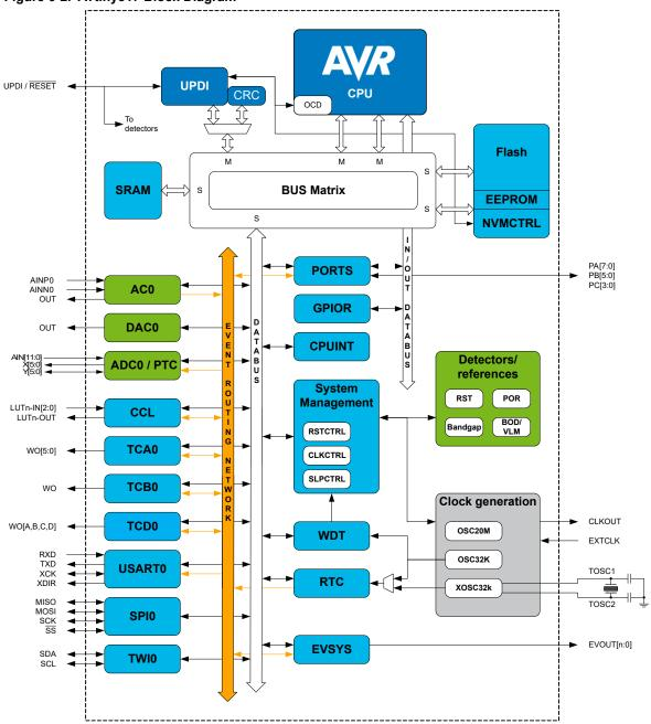
Figure 3-2. ATtiny817 Block Diagram
