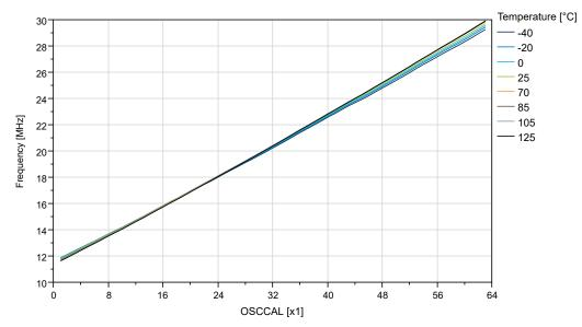
Figure 35-57. OSC20M internal Oscillator: Frequency vs. Calibration Value (V<sub>DD</sub>=3V)
