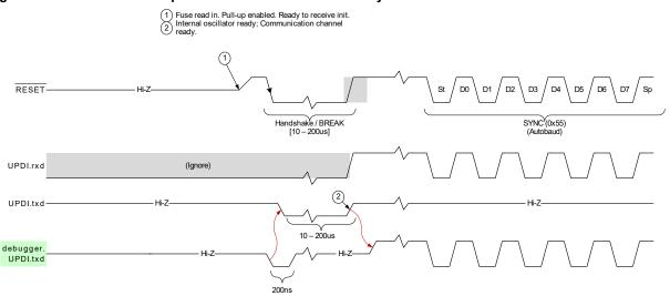
When the pull-up is detected, the debugger initiates the enable sequence by driving the line low for a minimum of 200ns and a maximum of 1us to ensure that the line is released from the debugger before the UPDI enable sequence is done.
