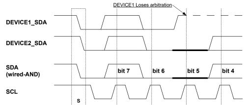
Figure 26-10 shows an example where two TWI masters are contending for bus ownership. Both devices are able to issue a START condition, but DEVICE1 loses arbitration when attempting to transmit a high level (bit 5) while DEVICE2 is transmitting a low level.
