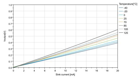
Figure 35-23. IO Pin Output Voltage vs. Sink Current (V<sub>DD</sub>=5.0V)
