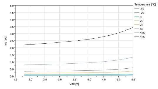
Figure 35-11. Power Down Mode Supply Current vs. V<sub>DD</sub> (all functions disabled)
