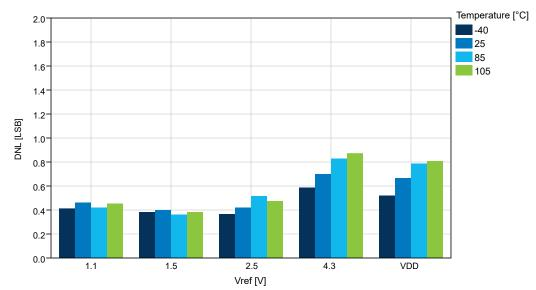
Figure 35-45. DNL vs. V<sub>ref</sub> (V<sub>DD</sub>=5.0V, 115ksps)
