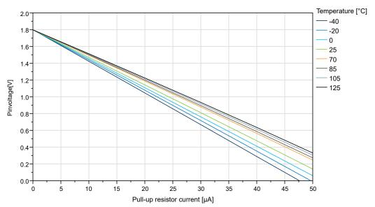
Figure 35-30. IO Pin Pull-Up Resistor Current vs. Input Voltage (V<sub>DD</sub>=3.0V)
