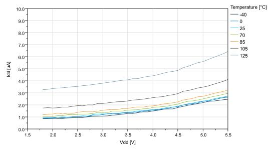
Figure 35-15. Standby Mode Supply Current vs. V<sub>DD</sub> (Sampled BOD running at 1kHz)
