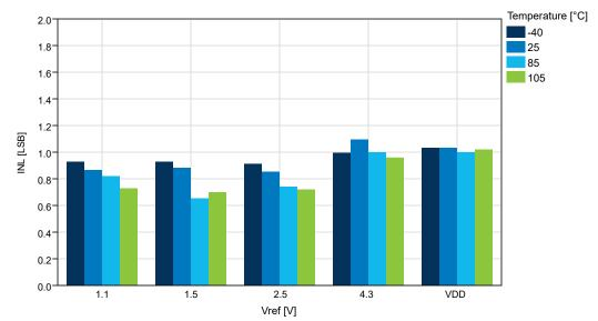
Figure 35-49. INL vs. V<sub>ref</sub> (V<sub>DD</sub>=5.0V, 115ksps)
