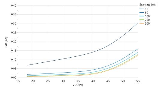
Figure 35-65. I<sub>DD</sub> vs V<sub>DD</sub> over Scanrates. Filterlevel = 16, T=25°C, Drift cal off.
