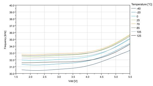
Figure 35-61. OSCULP32K Internal Oscillator Frequency vs. V<sub>DD</sub>
