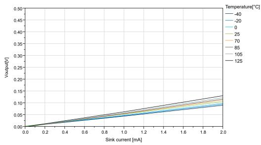
Figure 35-22. IO Pin Output Voltage vs. Sink Current (V<sub>DD</sub>=3.0V)
