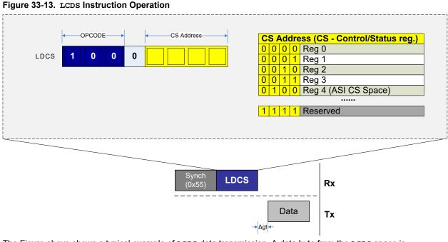
The Figure above shows a typical example of LCDS data transmission. A data byte from the LCDS space is transmitted from the UPDI after the Guard-Time is completed.
