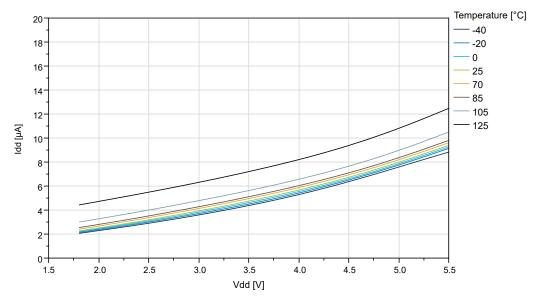
Figure 35-9. Idle Supply Current vs. V<sub>DD</sub> (f=32KHz OSCULP32K)
