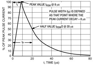
Figure 13. 8 X 20 µs Pulse Waveform
