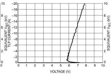
Figure 8. Negative TLP I-V Curve
