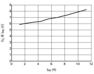
Figure 10. Negative Clamping Voltage vs. Peak Pulse Current (tp = 8/20  $\mu$ s)
