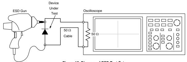
Figure 12. Diagram of ESD Test Setup
