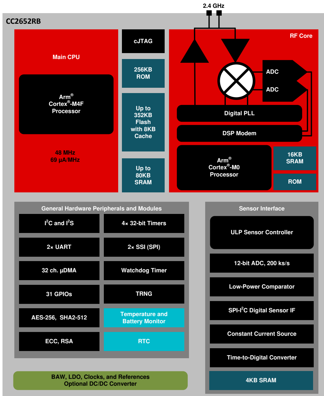
Figure 1-1. CC2652RB Block Diagram
