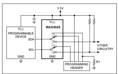
Figure 1. This analog switch (MAX4525) enables in-circuit programming by providing dual service for two lines (SDA and SCL) on the programmable device: for normal operation they connect to other circuitry, and for programming mode they connect to the programming header.
